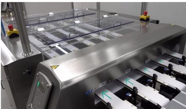
Figure 7 – Five-lane Checkweigher with Metal Detection
